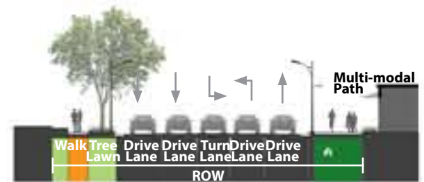
Section C-C: Conceptual section Near Inca Street
